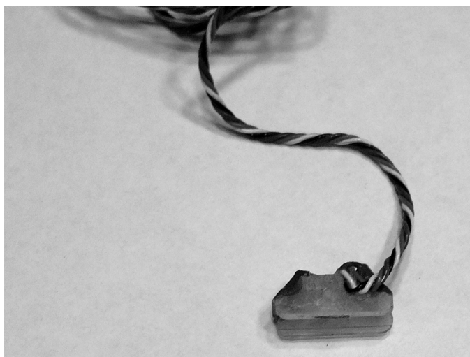
Fig. 3. An early prototype of a transit time flow probe, fabricated by Franklin, which contains two crystals on one side and a reflector on the other. This design was independently developed later by others and has become the industry standard.
