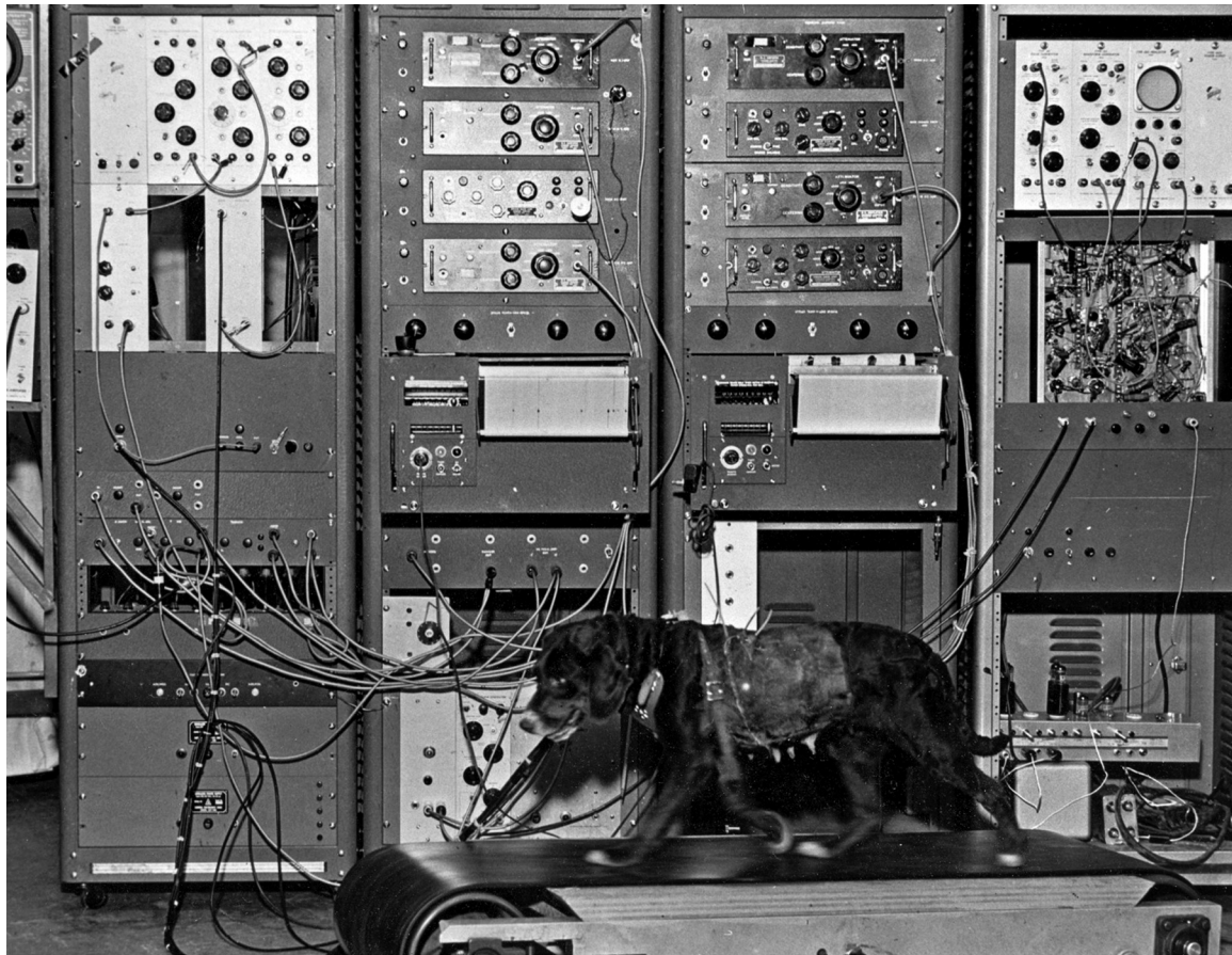
Fig. 2. A chronically instrumented dog exercising on a prototype Quinton treadmill at the University of Washington in the 1950s. The differential transit time flowmeter chassis on the right was mounted such that Dean Franklin could access the electronic components to deal with the severe drifting.
