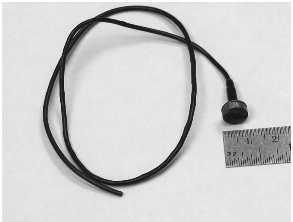
Fig. 7. One of the first prototype implantable pressure transducers that was used in the baboons and giraffes in Africa. Improved versions of this prototype subsequently became known as Konigsberg pressure transducers, which are still in use as of this writing.
